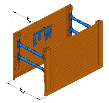
Adjust the struts to the desired trench width (fine adjustment).
