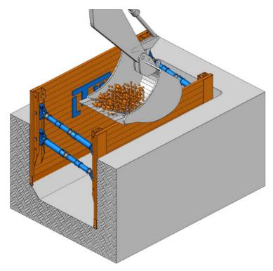
The shoring plates are to be pressed and not to be "hammered". For safety reasons it is not allowed to push or press on the struts and brace extensions.
