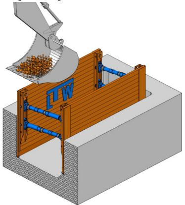
In order to protect the shoring plates we recommend using plate protectors.
