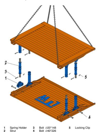
Place the Base Plate on the attachment points facing upwards.
