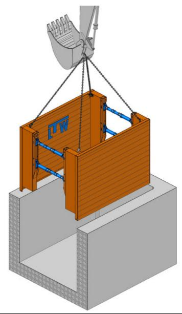
If the trench depths is greater than the Base Plate height, Base and Top modules must be assembled outside the trench and then inserted as a single unit into the trench.
