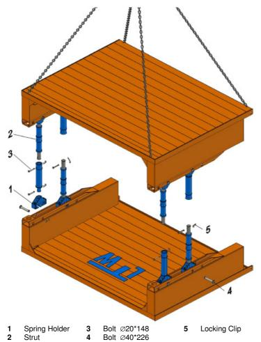
Place the Base Plate on the attachment points facing upwards.
