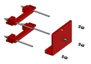
The clamping device engages behind the EG corner 3-sided and clamps the outside horizontal upper waler HEB 240. It creates a load-carrying connection which enables the forces that arise being discharged into the outer corner slide rails.
