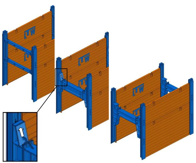
When assembling the H-Frame make sure that **the arrow is** in an upward position, in order to ensure the A-position.
