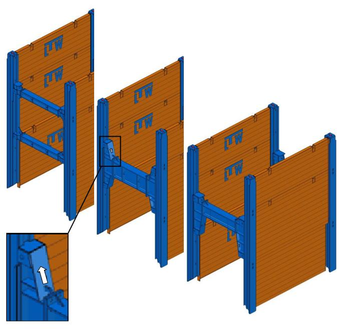
When assembling the H-Frame make sure that **the arrow is** in an upward position, in order to ensure the A-position.
